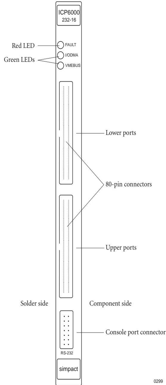
Figure 5-7: ICP Front Panel Showing Location of LEDs
