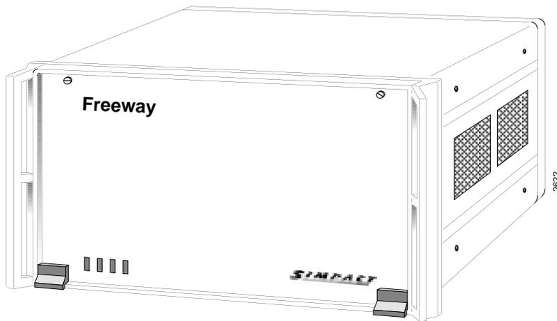
**Figure 2-1:** Front View: Freeway 4000 (with door closed)
