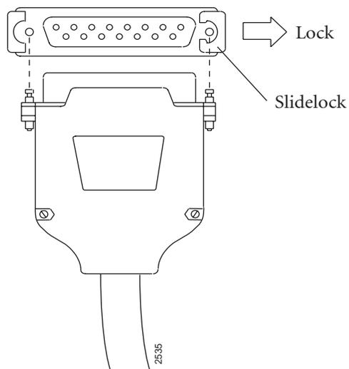
**Figure 2-5:** Slidelock on an AUI Connector
