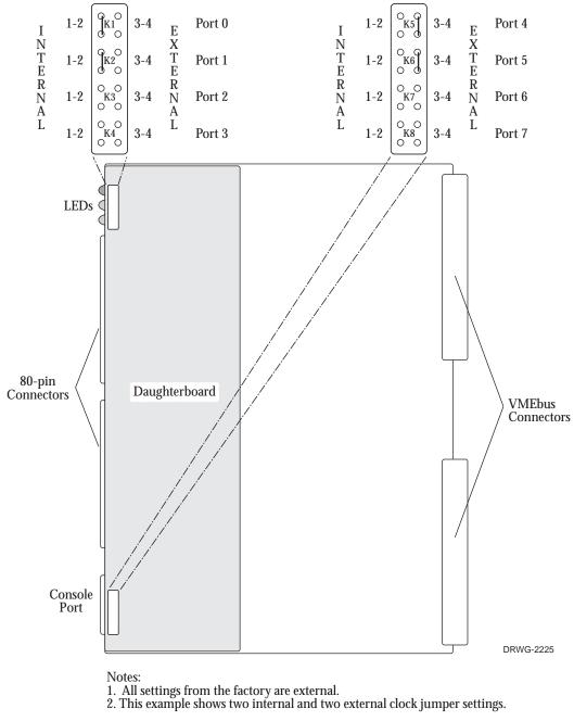
Figure C–1: 8-port V.35 Clock Jumper Settings
