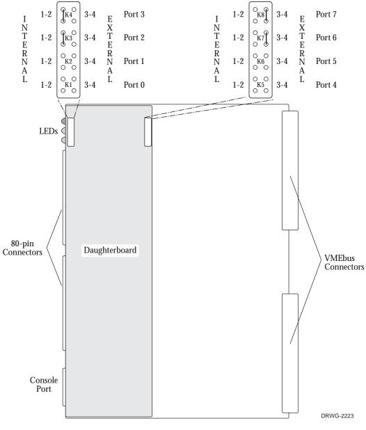
Notes: 1. All settings from the factory are external. 2. This example shows two internal and two external clock jumper settings.
