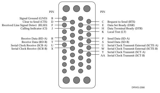
Signal suffixes -A and -B refer to differential signal pairs.
