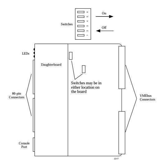
Figure 3–1: ICP6000(X)/ICP9000(X) Switch Settings
