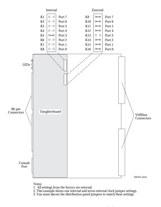
Figure B-1: 8-port MIL-STD-188C or EIA-232 Clock Jumper Settings
