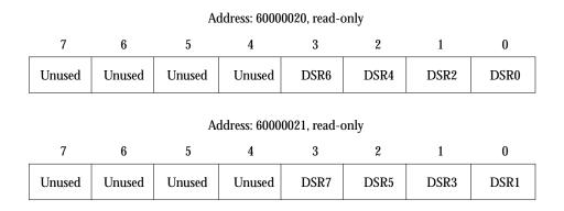
Figure B-2: Data Set Ready Address Decodes
