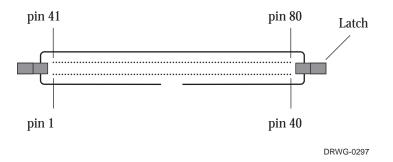
Figure A-4: Front View of 80-pin Connector on the ICP
