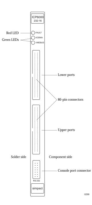
Figure 5–7: ICP Front Panel Showing Location of LEDs
