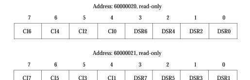
Figure C-2: Data Set Ready and Calling Indicator Address Decodes
