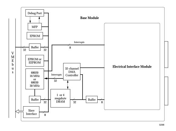
Figure 5–1: ICP6000(X)/ICP9000(X) Block Diagram
