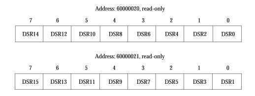
Figure A-2: Data Set Ready Address Decodes
