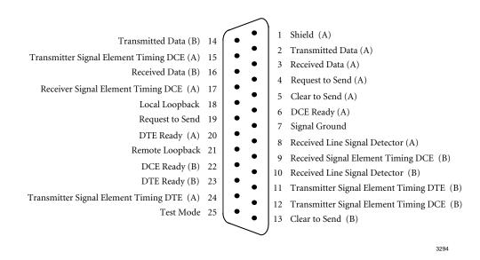
Figure 2: Signal Mapping for the 25-pin EIA-530 Interface
