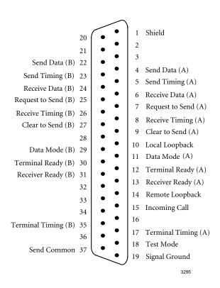
Figure 1: Signal Mapping for the 37-pin EIA-449 Interface
