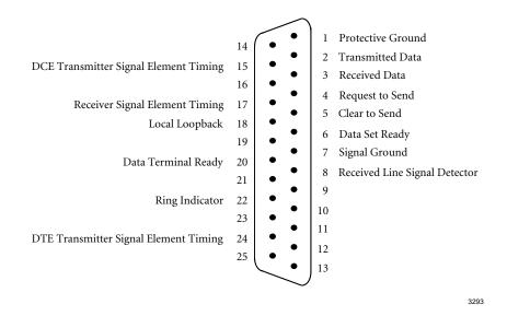
Figure 3: Signal Mapping for the 25-pin EIA-232 Interface
