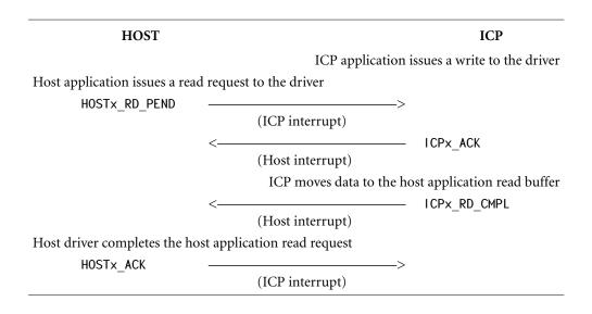
Figure 5–3: Host Reading Data from ICP
