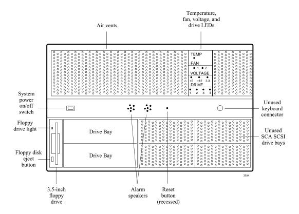
**Figure B–1:** Front Panel: Freeway 1300 (lockable door not shown)
