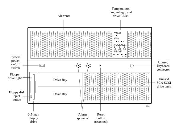
Figure 2–2: Front View: Freeway 1300 (lockable door not shown)
