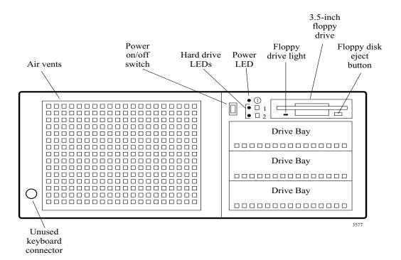
Figure 2–1: Front View: Freeway 1200 (lockable door not shown)
